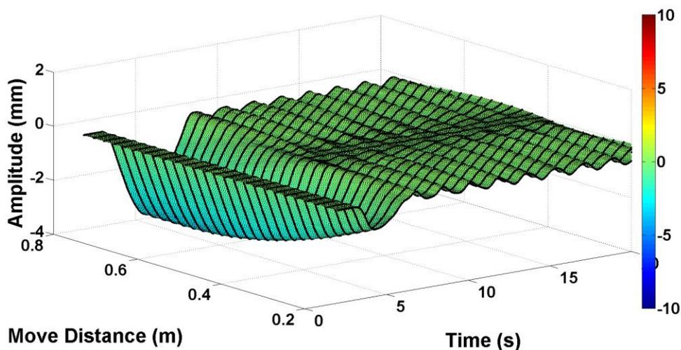
**Figure 4.** Variation in the Amplitude of Liquid Slosh with Move Distance using ZV shapers for  $\omega_0$ ,  $\omega_1$  and  $\omega_2$ , keeping the Liquid Depth at 42 mm and Suspension Length at 740 mm
