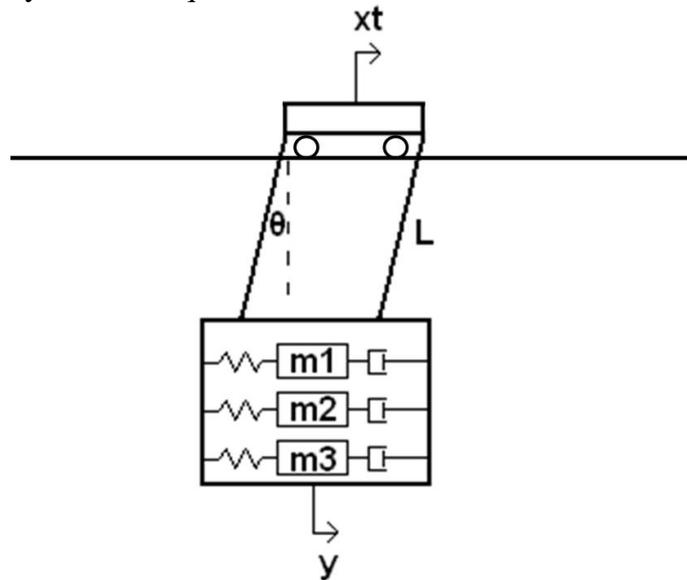
**Figure 1.** Schematic Drawing of Suspended Liquid Container
