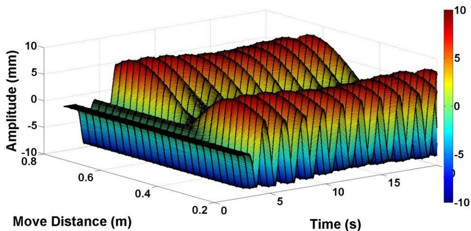
**Figure 3.** Variation in the Amplitude of Liquid Slosh with Move Distance using an Unshaped Velocity Profile, keeping the Liquid Depth at 42 mm and Suspension Length at 740 mm
