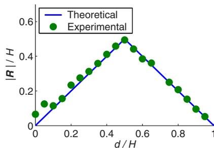
Fig. 11 Experimental and theoretical effects of dead-zone on ZV-shaped step commands
