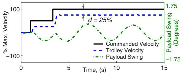
Fig. 10 Velocity command and system response for  $d=25\%$  maximum velocity
