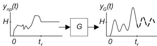
Fig. 3 Response of a harmonic oscillator to an arbitrary command
