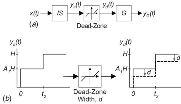
Fig. 2 Input shaping implemented on a system with dead-zone
