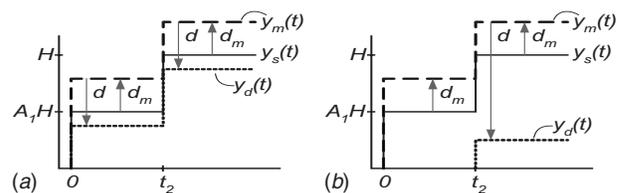
Fig. 13 ZV-shaped step command modified by dead-zone and inverse-dead-zone
