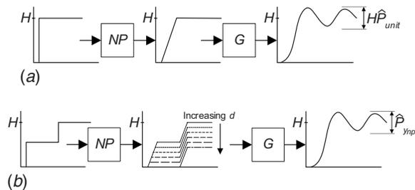
Fig. 8  $\hat{P}$ -values for a system with dead zone and rate limiting
