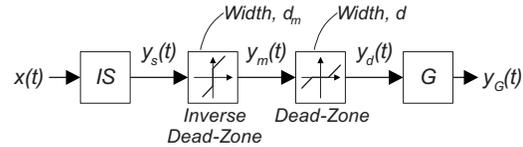
Fig. 12 Mitigation technique for eliminating the effects of dead-zone
