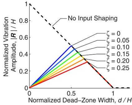
Fig. 4 Oscillatory effects of dead-zone on ZV-shaped and unshaped step commands
