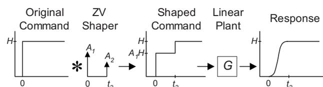
Fig. 1 Input shaping process
