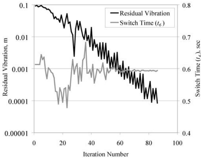
**Figure 5. Convergence and performance sensitivity results for UMZV<sub>O</sub> derivation routine**
