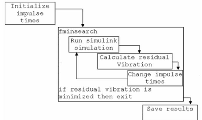
**Figure 4. Flowchart for UMZV<sub>O</sub> derivation routine**
