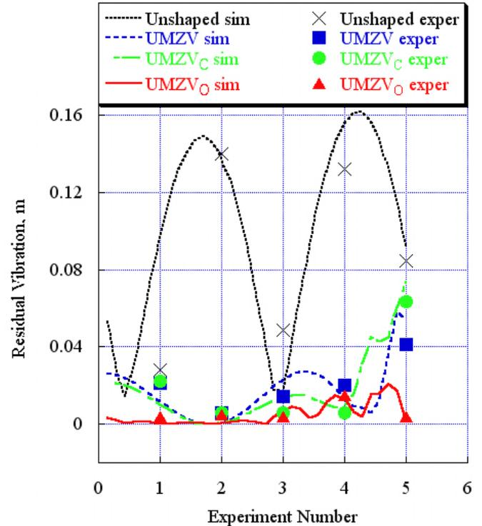
**Fig 10. Simulated and experimental responses of payload**
