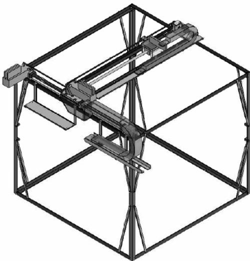
**Figure 2. Portable bridge crane experimental setup**
