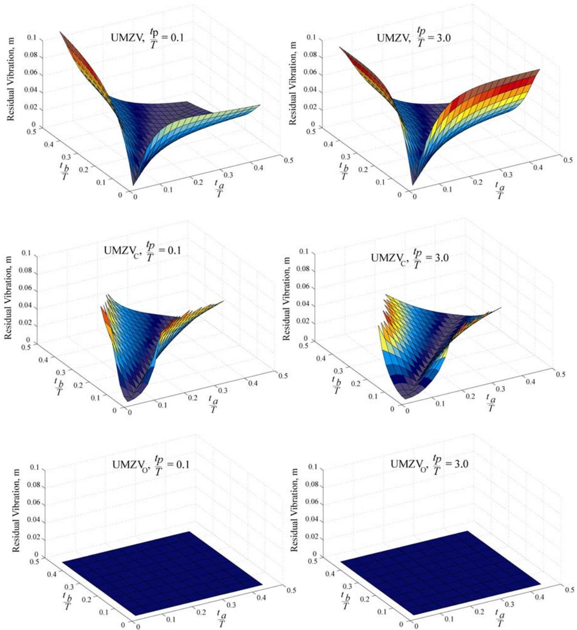
**Figure 8. Numerical comparison of simulated residual vibration for UMZV, UMZV<sub>C</sub> and UMZV<sub>O</sub> input shaped start-stop trajectories**
