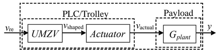
**Figure 3. Physical and functional (italics) block diagram of the portable bridge crane system**
