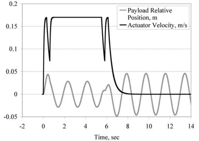
**Figure 6. Simulation results for UMZV<sub>O</sub> at iteration 1**
