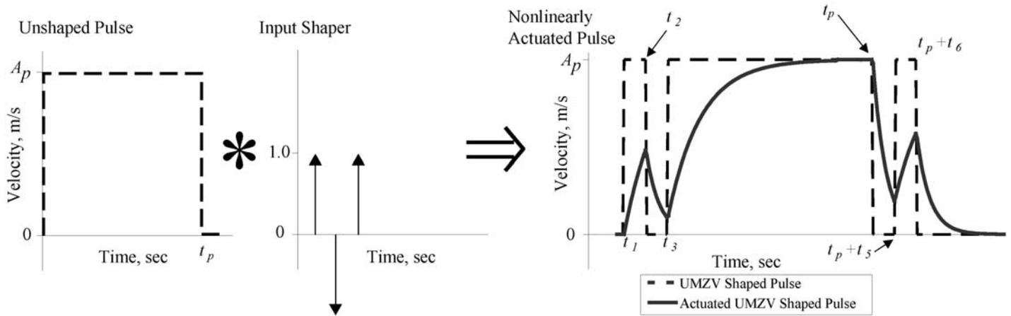
**Figure 1. Commanded and actual output from the non-linear actuator system**
