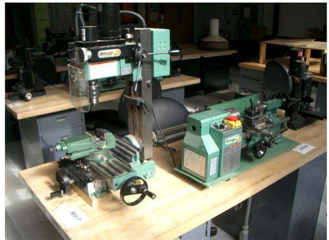
Fig. 3. Table-top Mill and Lathe.
