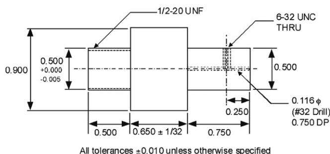
Fig. 5. Mechanical drawing of the coupler.
