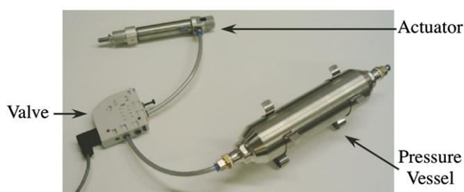
Fig. 2. The pneumatic components of the supply kit.
