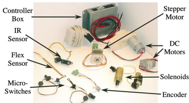
Fig. 1. The electro-mechanical components of the supply kit.
