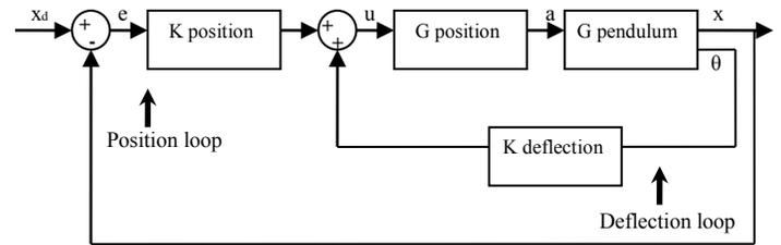
FIGURE 2. FEEDBACK LOOP SCHEMATIC
