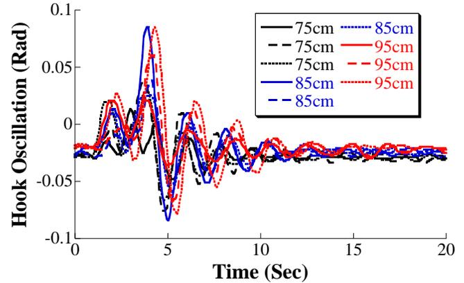
FIGURE 7. EXPERIMENTAL TRANSIENT RESPONSE FOR SELECTED HOIST LENGTHS
