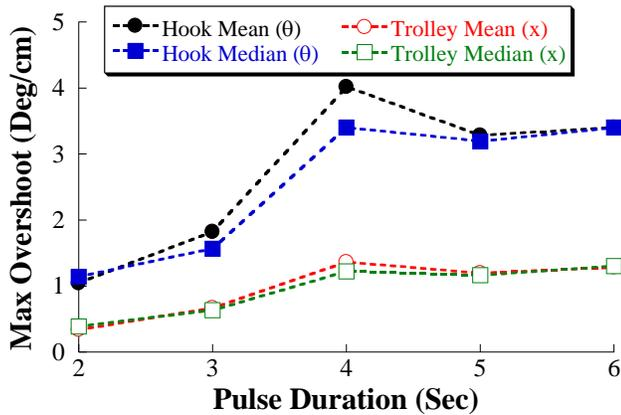
FIGURE 12: OVERSHOOT FOR VARYING WIND PULSE DURATIONS
