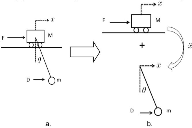
FIGURE 1. MODELS FOR BRIDGE CRANE ANALYSIS
