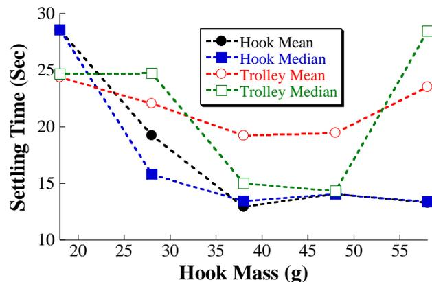
FIGURE 11: SETTLING TIME FOR VARYING PAYLOAD MASSES
