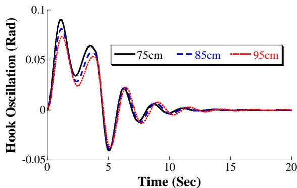
FIGURE 6. SIMULATED TRANSIENT RESPONSE FOR VARYING HOIST LENGTHS
