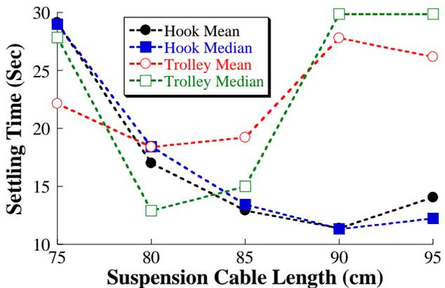
FIGURE 9. SETTLING TIME FOR VARYING HOIST LENGTHS
