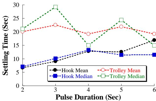
FIGURE 13: SETTLING TIME FOR VARYING WIND PULSE DURATIONS
