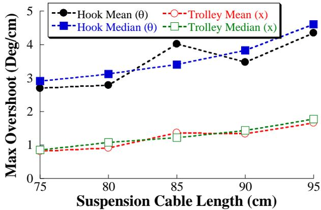
FIGURE 8. OVERSHOOT FOR VARYING HOIST LENGTHS
