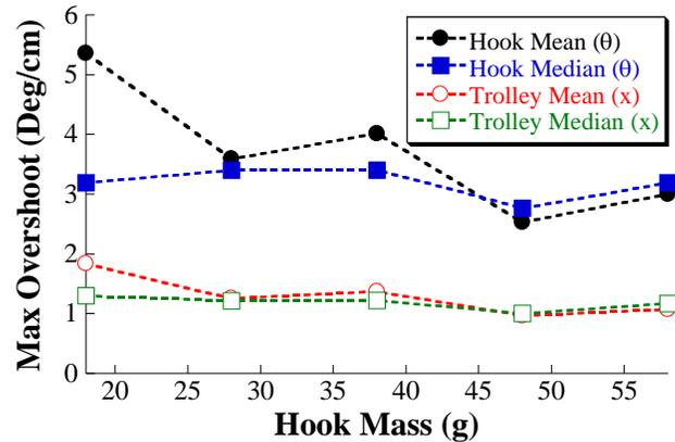
FIGURE 10. OVERSHOOT FOR VARYING PAYLOAD MASSES
